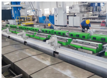
Milling of rail points
